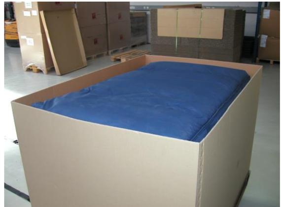
**Fig 2) Thermal blanket used for loading cargo in LD9 container**
