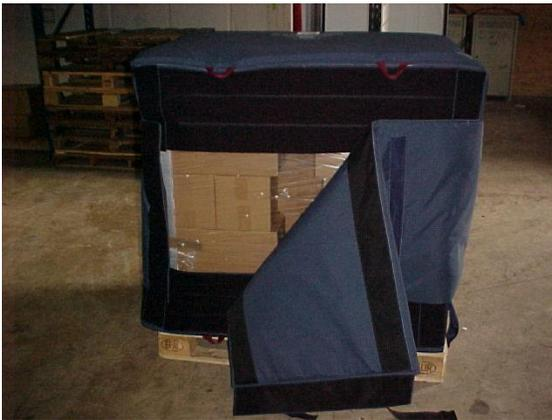
**Fig 1a) Thermal blanket used in pallet box**
